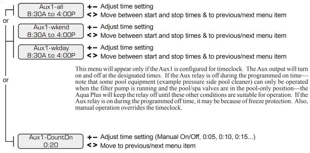
This menu will appear only if the Aux1 is configured for countdown timer. This setting is the time after you manually turn on the Aux relay until the Aqua Plus automatically turns off the relay. You can also manually turn off the relay at an earlier time by pressing the AUX1 button.
