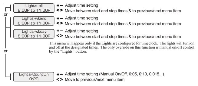
This menu will appear only if the Lights are configured for countdown timer. This setting is the time after you manually turn on the lights until the Aqua Plus automatically turns off the lights. You can also manually turn off the lights at an earlier time by pressing the LIGHTS button. If the Lights relay is on during the programmed off time, it may be because of freeze protection.
