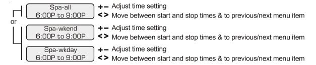
This menu is only available if the system has been setup for "pool and spa". During the programmed spa time, the Aqua Plus will turn on the filter pump and move the pool/spa valves into the "spa-only" position. The heater will automatically heat the spa up to the programmed spa temperature (page 7). This programmed spa operation will take precedence over all other automatic functions, only manual operation of the filter button or pool/spa valve button will override this function.
