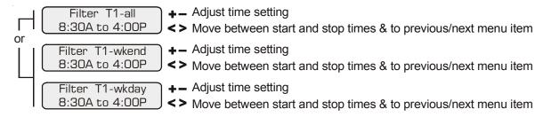
For one speed pumps, this is the first filter timeclock and will determine the normal hours of filtration for the pool. For pool/spa combination systems with spillover enabled, the valves will automatically switch to spillover mode at the start of the filtration period. For all other systems, the valves will switch to the pool-only position. Refer to the text above for general notes regarding timeclock programming.
