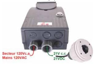
The supply box must be powered using 120V single phase current with 60Hz, and protected by a class A differential device (ground fault circuit interrupter (GFCI)), capable of providing a sufficient intensity (2A min). The cable section used for the supply must be suitable and functional over its entire length.
