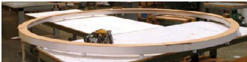
12' concave circle sheeting waterfall feature with bottom inlets.
