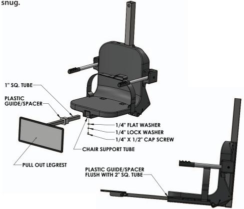
The PULL-OUT LEGREST is now ready to use. However, before using, slide the legrest in and out, and put the pad up and down to make sure everything works smoothly.
