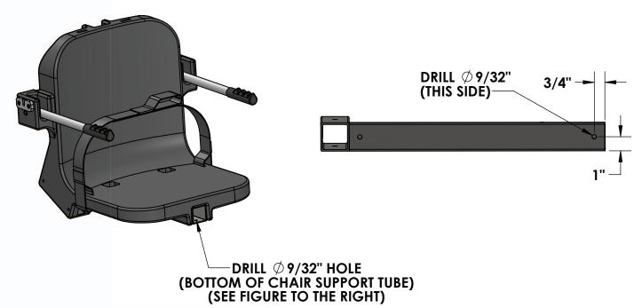
3. Orient the pull out legrest as shown below and slide the plastic guide/spacer into the chair support tube. Tap the palstic guide/spacer with a hammer or mallet until flush with the end of the support tube. The threaded hole in the bottom of the plastic guide/spacer should line up with the hole drilled in the support tube. Install the washers and 1/4"-20 x 1/2" cap screw from underneath and tighten until snug.
