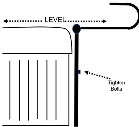
3. Ensure that all other screws and bolts are firmly tightened.
